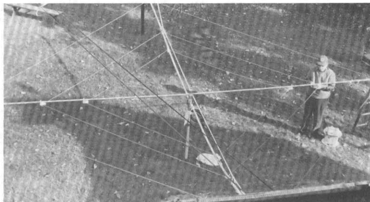
Fig. 9 -- Each element is tuned in a horizontal attitude and mounted on temporary poles 8 feet above the ground.
